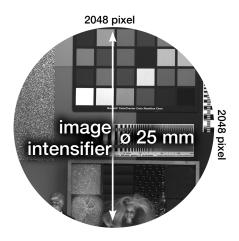
The projected image circle is completely covered by  $2048 \times 2048 \times 6.5 \mu m$  pixels of the sCMOS detector. There is no "waste" of valuable intensifier area. As a consequence the four corners of the sCMOS sensor remain black. For a fast scan of just a few vertically centered lines - the camera module allows you to achieve more than 56,000 fps for such a ROI - the full line length of 2048 pixels is available.
