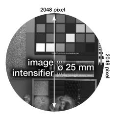
The projected image circle is completely covered by 2048 x 2048 6.5 µm pixels of the sCMOS detector. There is no "waste" of valuable intensifier area. As a consequence, the four corners of the sCMOS sensor remain black. For a fast scan of just a few vertically centered lines – the camera module allows you to achieve more than 7000 fps for such a ROI - the full line length of 2048 pixels is available.
