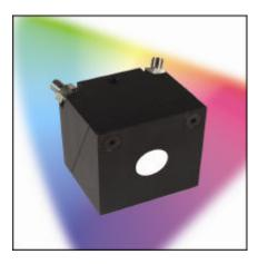
The **StellarSphere IC2** is a 2" cube with internal integrating sphere. It has a 5/8" input port, internal reflective coating, and SMA fiber optic output. The additional SMA input can be used for reflectance illumination.
