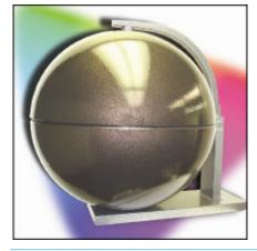
The **StellarSphere IS12** is a 12" integrating sphere that opens to allows for simple internal mounting of devices for light measurement such as discrete LEDs, arrays, and more. A tungsten halogen bulb and data file are included for system calibration using the SpectraWiz® radiometer software.
