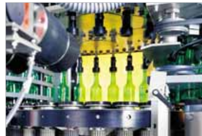
Bottle inspection measuring at a high dynamic range, courtesy of Kronen AG, Regensburg, Germany
